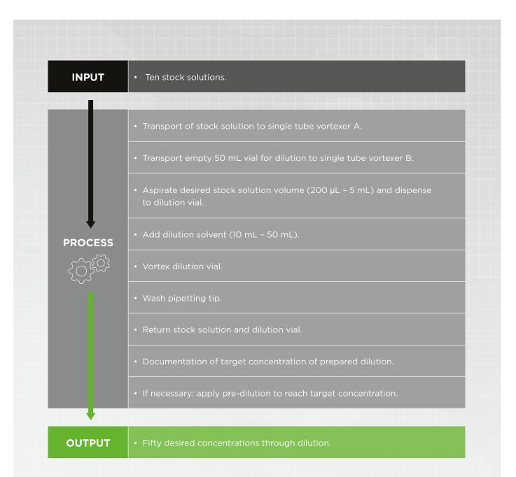
With this process a throughput of **160 dilutions in an 8 h working day** is achievable with a preparation time of maximum **180 seconds per dilution**.
